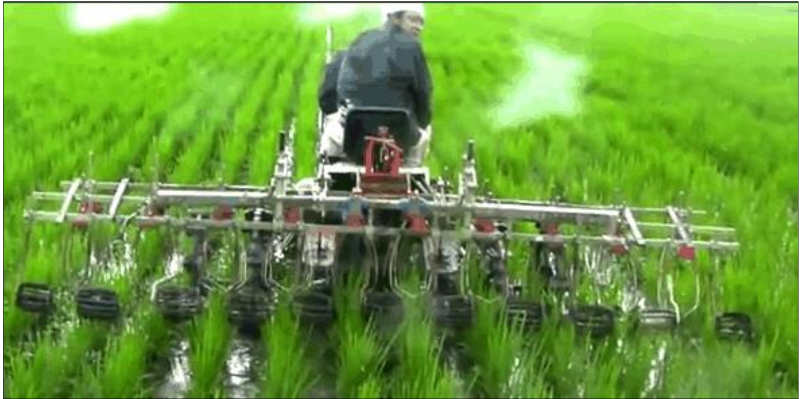
11-Row Rotary Weeder Behind Transplanting Tractor
